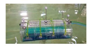
Asturmadi Reneergy numerically tested a device to harvest solar energy in the marine environment in collaboration with the University of Oviedo. The device consisted of a top-of-pole mount that holds the solar panels and a tension leg platform (TLP) that keeps the structure afloat while restricting its motions. The testing concluded in February and the results were very promising.
